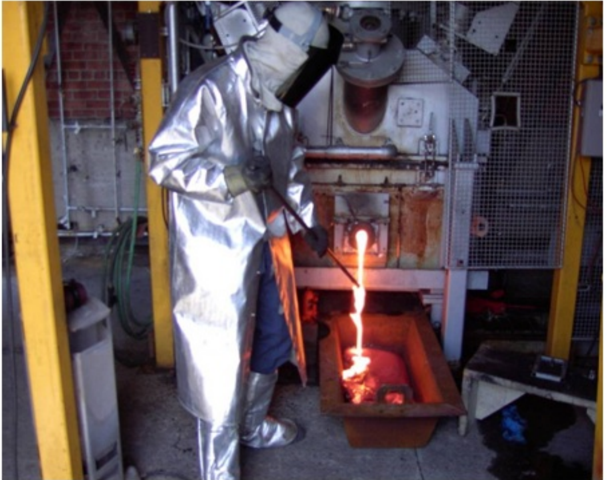
Picture 1: Molten slag pouring from plasma waste gasification reactor ( Pyrogenesis Inc , Montreal, Canada)
