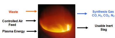
Figure 1: Plasma gasification process flow chart
