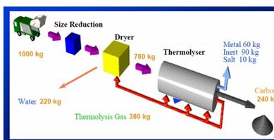
Figure 1: Pyrolysis process flow chart
